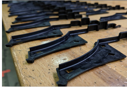
Fortify Digital Tooling insert and molded parts for an automotive application.
